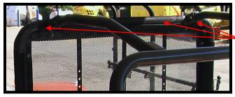
1. Wrap the velcro around the rear top bar on the roll cage. Ensure that the end flaps are secured around the bar as shown in the pictures.
