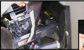
5. Locate the strap on the passenger side with the adhesive velcro strip. Clean the plastic panel on the vehicle with alcohol, remove the strip and secure to plastic panel as shown.
